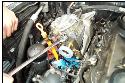
Figure 9 – Use a 24mm Open End Wrench to Remove the Fuel Supply Solenoid Valve
