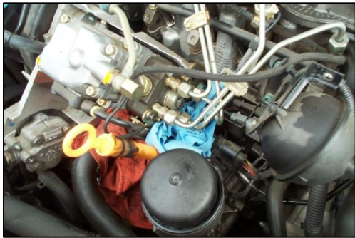
Figure 3 - Paper Towels Under the Injection Pump
