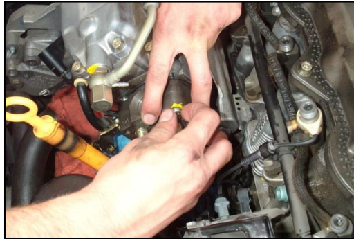
Figure 35 - Thread the Topmost Torx Screw Back into the Pump Head
