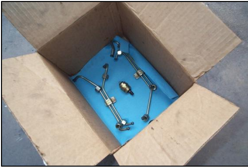
Figure 12 - in the Box with the Injector Lines
