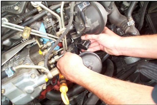
Figure 14 - Unplug the Injection Pumps 8 or 10 Pin Plug
