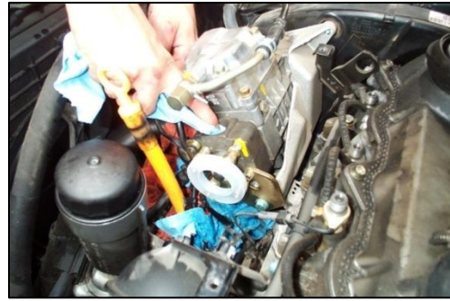
Figure 13 - Carefully Wipe Away Any Dirt from Around the Edges of the Fuel Cutoff Solenoid Orifice by Wiping from the Center of this Hole Outward
