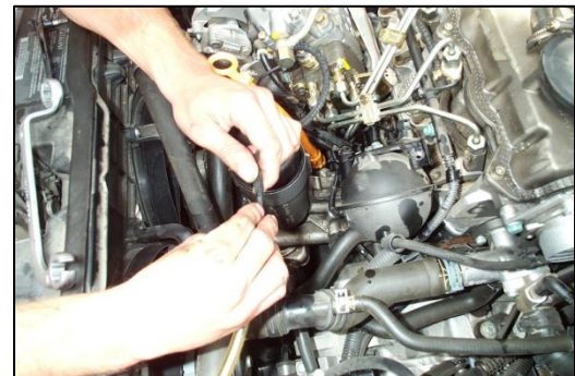
Figure 40 – On the Exposed Nipple of the T-Fitting
