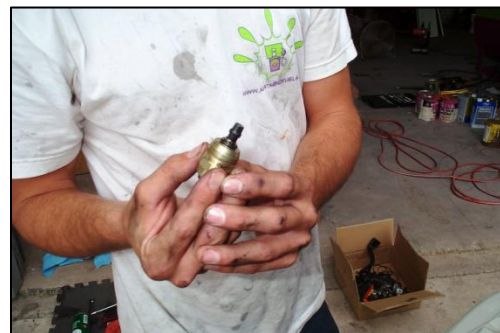
Figure 11 - Set the Solenoid (with Plunger) Aside in a Clean Place
