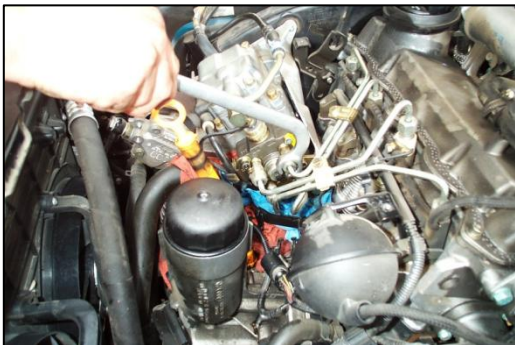
Figure 5 - Remove the Hard Metal Injector Lines with a 17mm Flare Wrench
