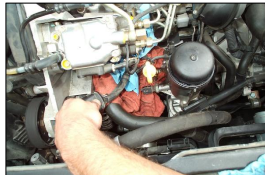
Figure 17 - Pull the Pump-Side Part of the Wiring Harness Forward and Then Toward the Timing Belt Side
