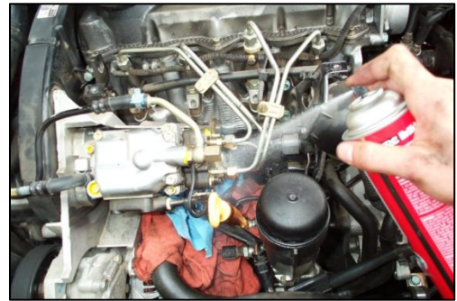
Figure 4- Spraying Brake Cleaner On All of the Fittings
