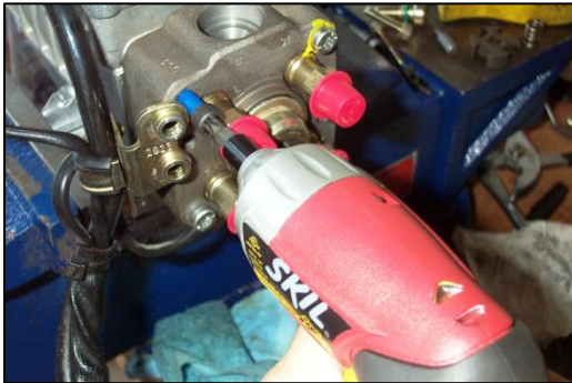
Figure 25 - Replace It with the 55mm Long Allen Screw
