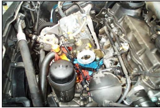
Figure 7 - Place the Opaque Plastic Ring or Red Plastic Caps over the Injector Output Valves
