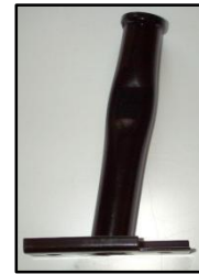
Figure 49 - The post is not welded perpendicular to the base plate
