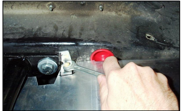
Figure 80 - Tighten the 10mm headed bolt on the driver side panel but likewise don't go crazy with it since it is going into a 6mm aluminum threaded hole
