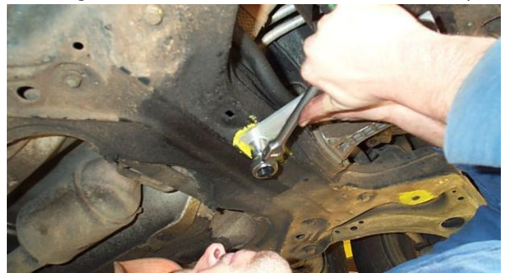
Figure 40 - The rivnut will mushroom out and expand
