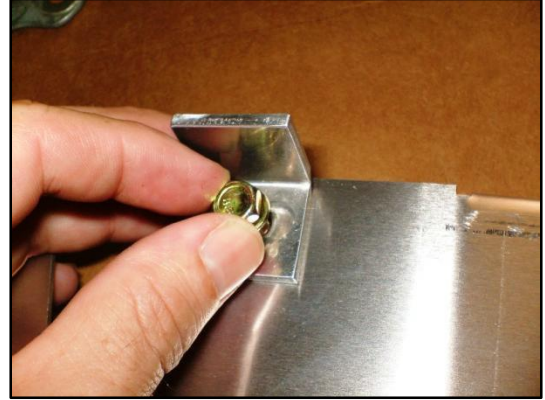
Figure 59 - Thread the supplied 6mm bolt through the small bracket and into the threaded insert
