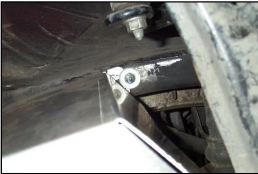
Figure 60 - Slip the rear mounting tab's open slot onto the stud
