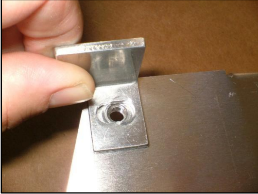
Figure 58 -Place the small angle bracket from the parts bag against the side panel
