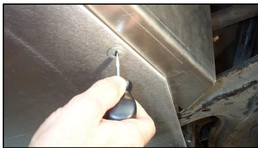
Figure 75 - Turn the screw 90 degrees clockwise with your stubby or regular length flat head screwdriver
