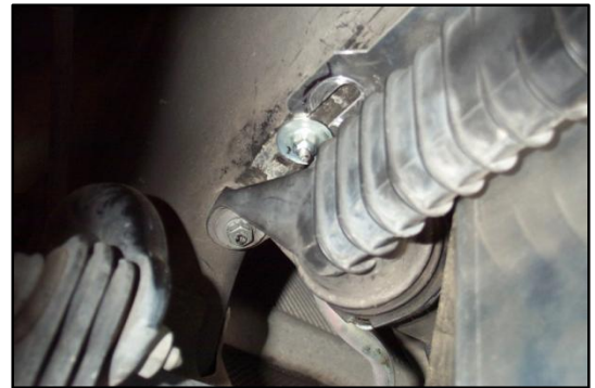
Figure 67 - Engage the rear mounting slot onto the frame rail stud
