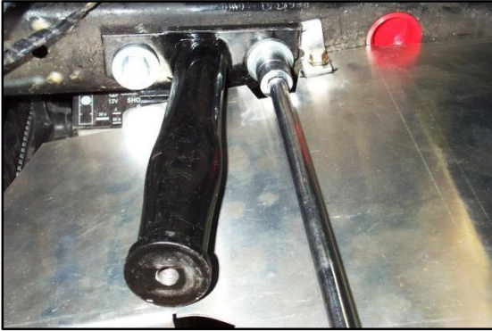
Figure 77 - Tighten all four of the front mounting post bolts to 20 ft.-lbs using your 12 inch long extension and 17mm socket
