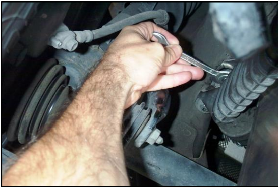
Figure 77 - Tighten all four of the front mounting post bolts to 20 ft.-lbs using your 12 inch long extension and 17mm socket
