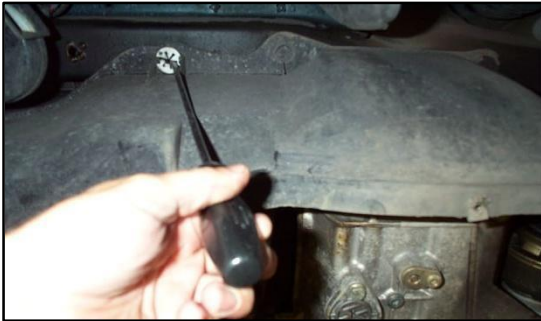
Figure 28 - Place a flat bladed screwdriver in one of the star nut's radial slots
