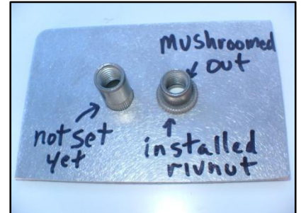
Figure 35 - Rivnuts are locked into the body by setting them
