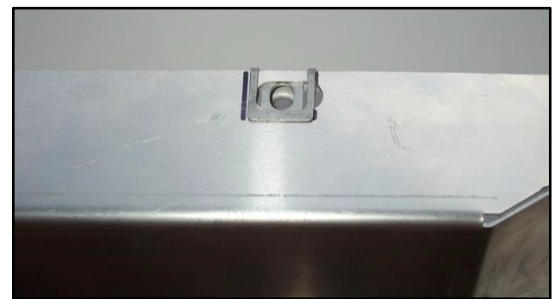
Figure 76 - You can slide the side panel's Dzus receptacle left or right in its slot if it is not where it needs to be
