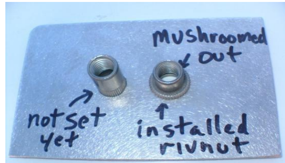
Figure 40 - The rivnut will mushroom out and expand
