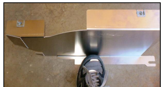
Figure 57 - Both clips properly installed on the passenger side panel
