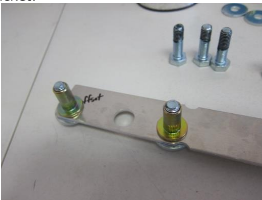
Figure 44 - Insert the bolts through the rivnut tool on the side opposite of the stamped letters
