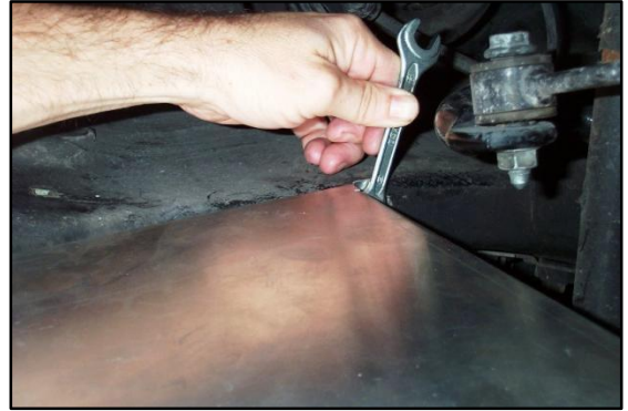
Figure 78 - Finish the tightening the left side sheet metal nut with a short open end 10mm wrench
