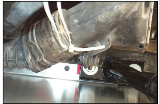
Figure 71 - The double tab can be slid in between the mounting post and frame rail
