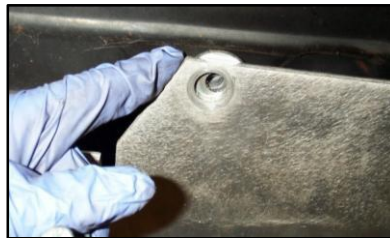
Figure 73 - The last extra washer between the skid plate and the rear center bolt hole
