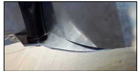
Figure 74 - Slide the driver and passenger side panels forward or rearward until the top of the curved section matches up with the curvature of the skid plate
